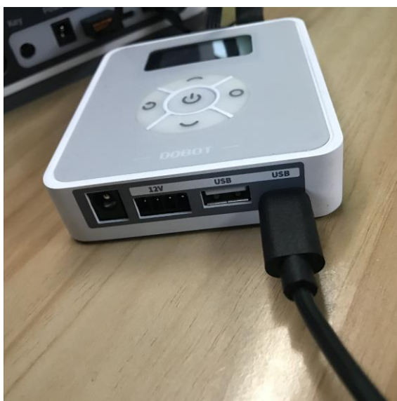
Figure 2.5 Connect Magician Lite to the electrical outlet
