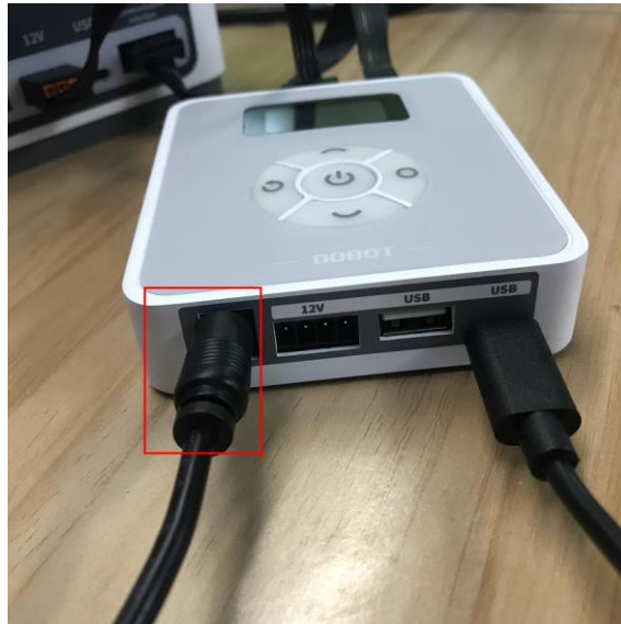
Figure 2.6 Connect power adaptor
