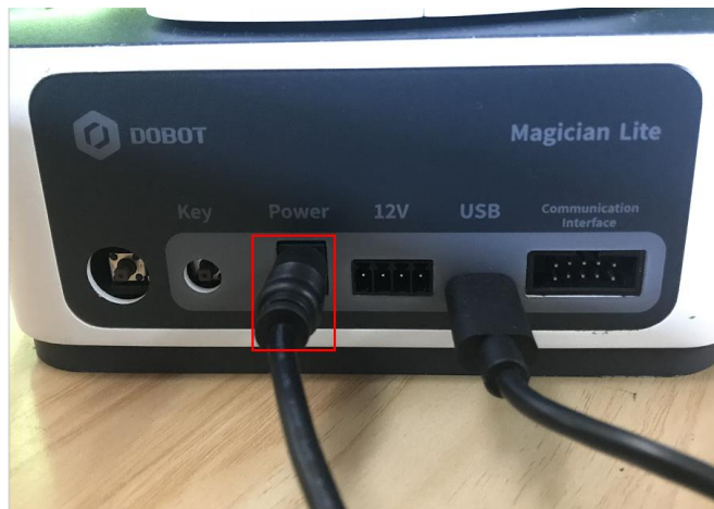
Figure 2.3 Connect Magician Lite to the electrical outlet
