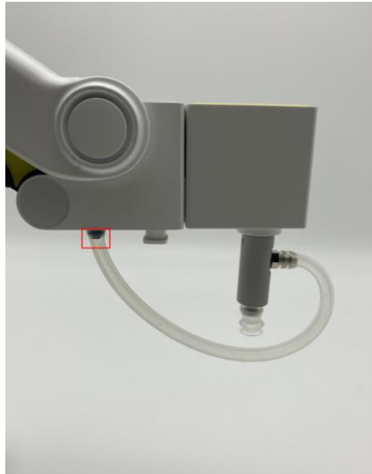
Figure 5.10 Install an air tube
