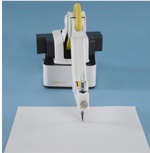
Figure 5.51 Adjust the position of the pen nib
