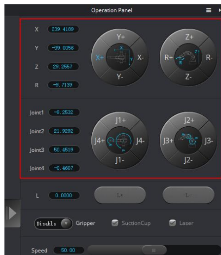
Figure 2.20 Jog Magician Lite in the Cartesian or Joint coordinate system
