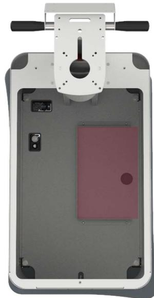
Place the controller in the marked area with the door faced like shown.
