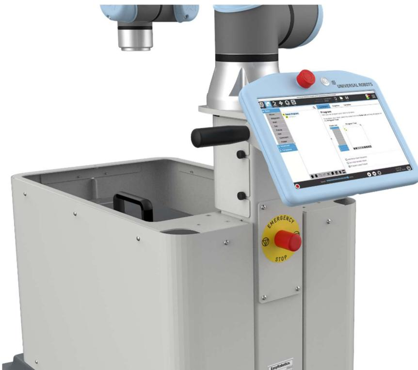
Mount the teach pendant and place the cable through the slot beside the robot.
